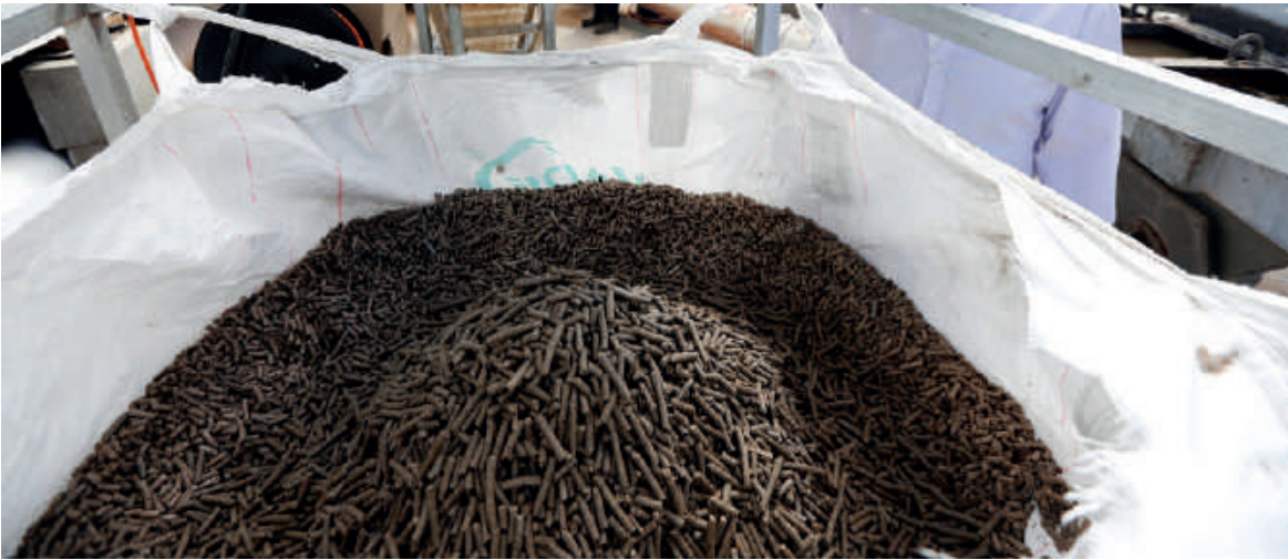
Pellets of cellulose fibre recovered from sewage. These pellets, marketed under the name Recyllose, can be used as fuel or in producing paper, insulation, construction materials and bioplastics. Photo: Reuters / Baz Ratner
