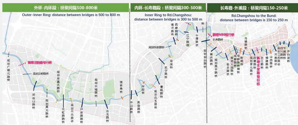
Figure 38 The planning of bridges crossing Suzhou Creek (Shanghai Planning and Land Resource Administration, 2018)
