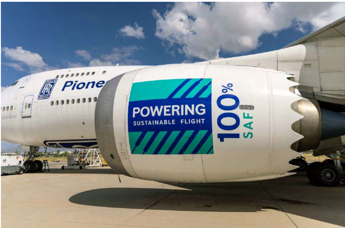
Rolls-Royce Trent-1000 engine operating with 100% SAF on a Boeing 747-200 Flying Test Bed.
