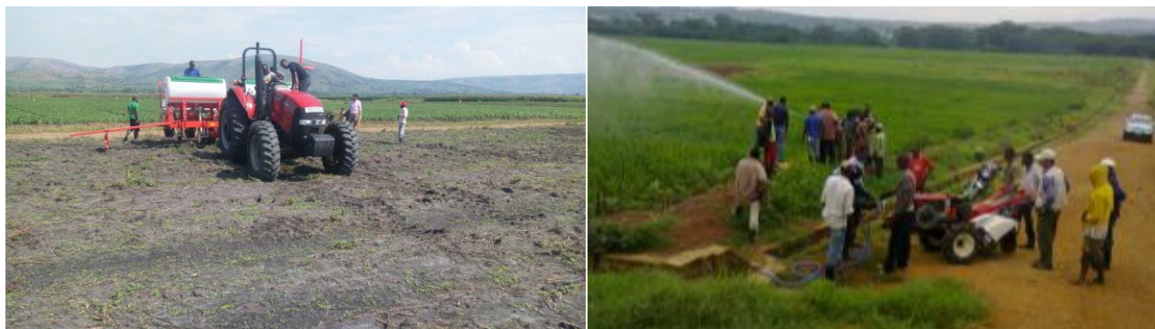
(a) Boom sprayer attached to four-wheel tractor at the KABOKU cooperative farm (b) Two-wheel sprayer Muvumba rice marshland
