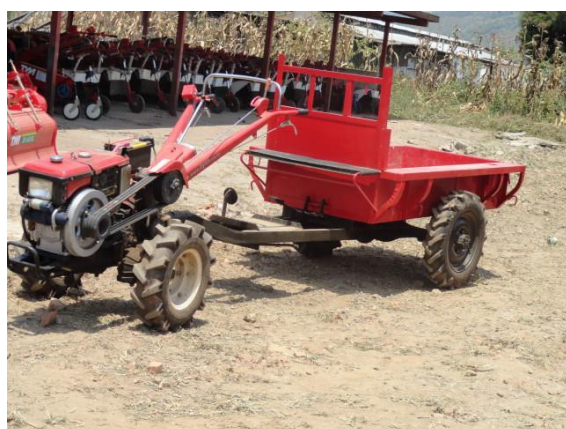
(a) Two-wheel power tiller attached to a trailer
