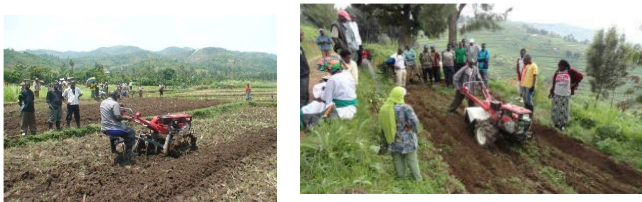
(a) Land preparation: Power tiller plowing land with disc plough (b) Land preparation: Power tiller plowing land with moldboard plow
